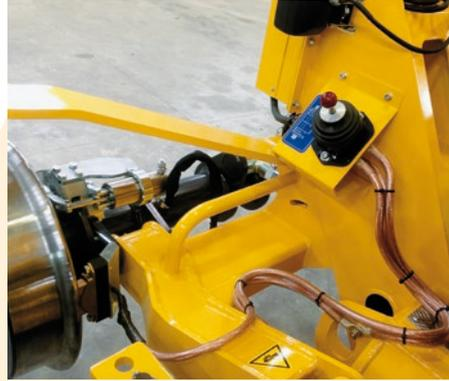
Equipotential bonding according to **RIS1530**
